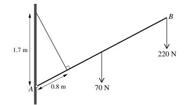
A uniform beam AB has length 2 m and weight 70 N. The beam is hinged at A to a fixed point on a vertical wall, and is held in equilibrium by a light inextensible rope. One end of the rope is attached to the wall at a point 1.7 m vertically above the hinge. The other end of the rope is attached to the beam at a point 0.8 m from A. The rope is at right angles to AB. The beam carries a load of weight 220 N at B (see diagram).
